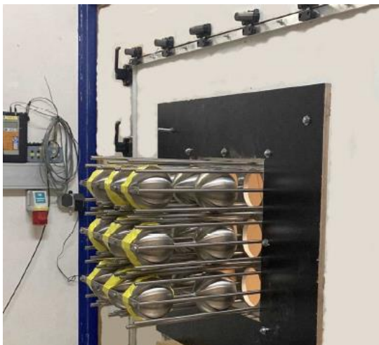
Figure 5 TFP system pressure drop test
